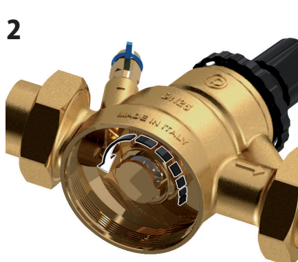
2 With an 32mm socket unscrew the \Delta P regulator
